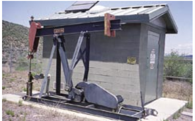
Figure 12—Solar-powered jack pump.
