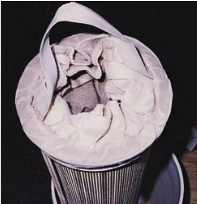
Figure 76—Used bag filter in support basket.
